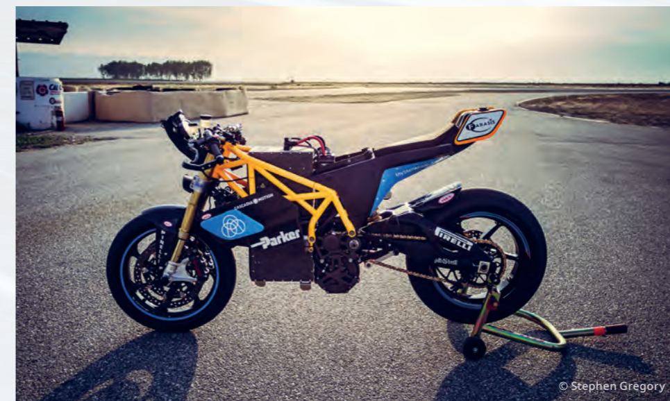
With bodywork removed, the central location of the battery in the Lightfighter frame is visible
